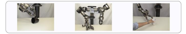
Fig. 1. Potential Maniplations faults. (left) Missed grasp. (middle) Heavy object. (right) Uncontrollable obstacle.
