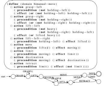
Fig. 2. Example grasping domain for bimanual manipulation and the corresponding policy automaton. Faults include failed grasps, heavy objects require lifting with two hands, and limits which require stopping the motion.
