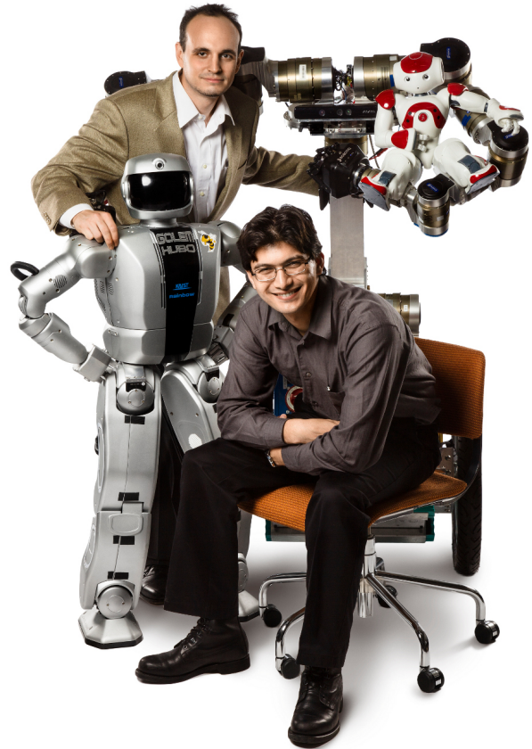
Fig. 1. Hubo, Golem Krang, and NAO: Existing Robotic Systems where Ach provides communications between hardware drivers, perception, planning, and control algorithms.
