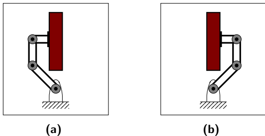
Figure 5. Example object placements that cause disconnected post-configurations by “blocking-in” the robot. For this 3-DOF planar robot, the two sides of the workspace are disconnected.
