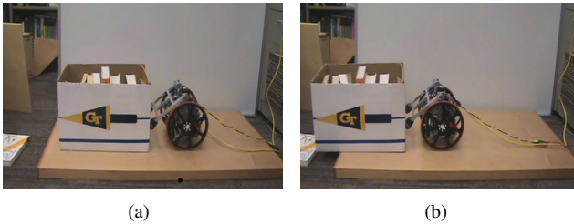
Fig. 8. Sparky pushing a box full of books weighing 6 Kg using the simple push strategy.
